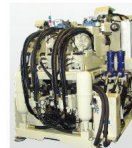
ACC高速射出機裝置及全閉環油電路 Accumulator for high speed injection, and injection closed loop system
